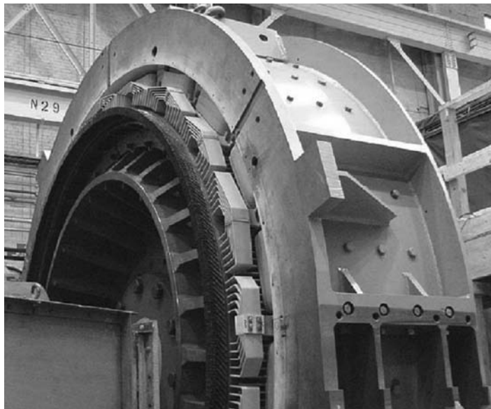
FIG. 6-2 Stator of a 375 kW dc motor. Courtesy of General Electric
